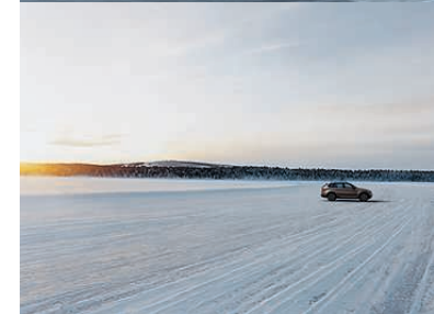
The low frictional coefficients on the frozen lakes are perfect for repeatable test drives at the limits of adhesion.
