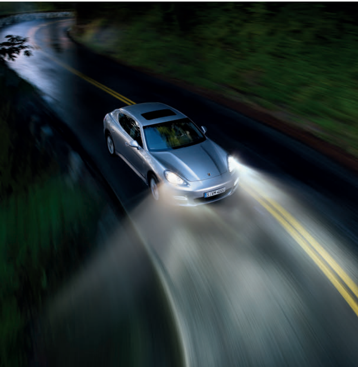
Cornering lights of the Porsche Dynamic Light System (PDLS)
