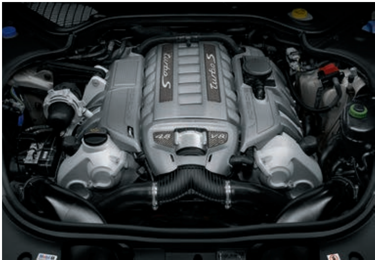
The twin-turbo V8 engine in the Panamera Turbo S
