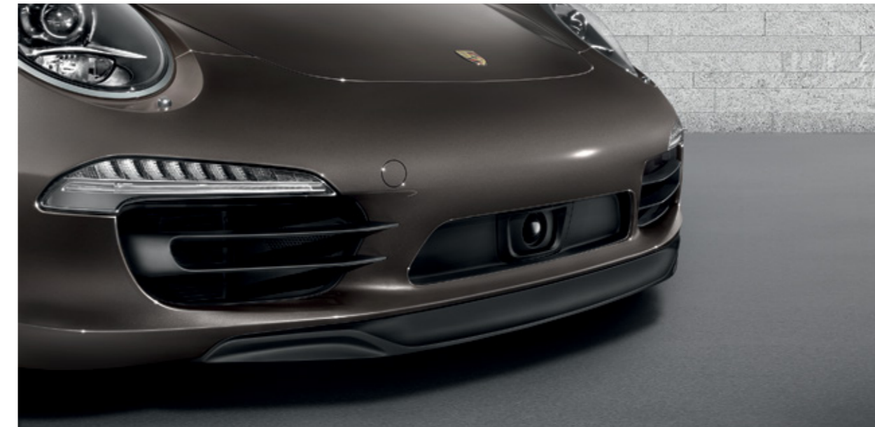
Radar sensor of adaptive cruise control
